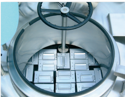
Three Biosystem 40 units provide fully automated storage for over 44,000 specimens each in vapour phase with dependable temperature stability at -185°C (Plus/minus 4°C)
